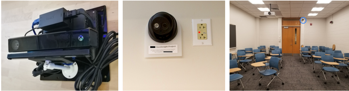
Fig. 2. Left: Early version of EduSense, using a Microsoft Kinect One depth camera and Intel NUC. Center: Current system, which uses networked 4K cameras that are accessed from a central serve. Right: example classroom from our deployment with instructor-facing camera circled in blue.
