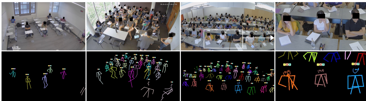
Fig. 4. Top row: Example classroom scenes processed by EduSense (image data is not archived; shown here for reference and with permission). Bottom row: Featurized data, including body and face keypoints, with icons for hand raise, upper body pose, smile, mouth open, and sit/stand classification.
