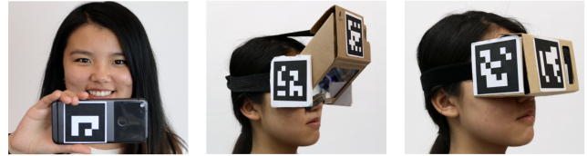
Figure 3: BodySLAM works across different AR/VR modalities, including mobile "passthrough" AR (left), head-worn AR (center; HoloKit), and VR (right; Google Cardboard).
