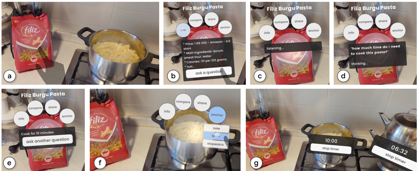
Figure 1: XR-OBJECTS allows users to (a) select and interact with real-world objects in AR as if they were digital objects. Automatically generated object-based AR context menus allow objects to (b) provide information about themselves, such as nutritional facts and ingredients. For example, a user (c, d, e) asks a question about the cooking time of pasta, and then (f, g) uses the answer to set a spatial timer widget anchored to the relevant pot in 3D space.
