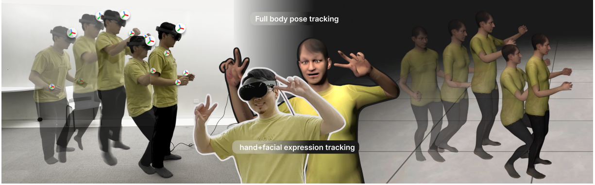
Figure 1: FlowAvatar: a unified system for real-time full-body pose tracking, hand and facial expression tracking, and personalized look-alike appearance on consumer XR devices.
