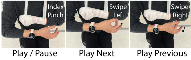
Figure 11: EI-Lite for accessible smartwatch control. A user with limited hand functions performs one-handed micro-gestures to control a smartwatch.
